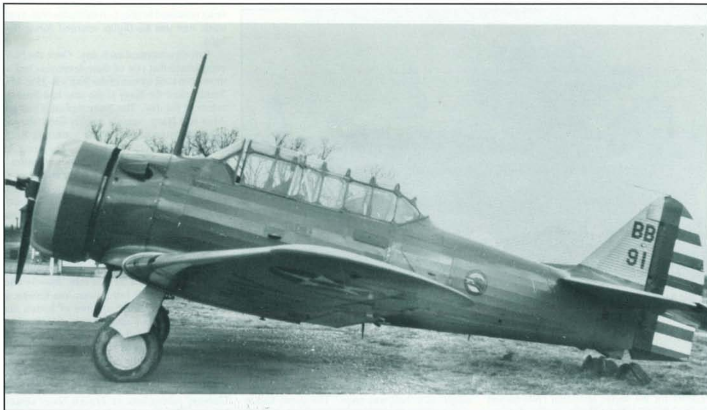
While similar to the North American AT-6 Texan, the BC-1s had a larger rudder and an oil cooler vent located higher on the left side of the forward fuselage. This Blue and Yellow ship carried the BB tail code for the 2nd Bombardment Group and the 49th Bomb Squadron insignia on the waist. These aircraft were used for administrative transportation. (Courtesy of the United States Air Force/Air Combat Command Historian)
