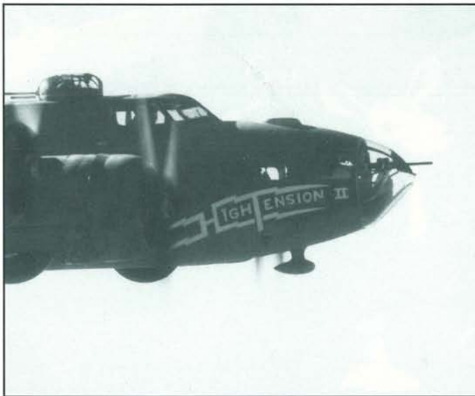
"High Tension II". Note modified nose section with single 50 caliber machine gun firing forward. (Courtesy of Photo Section/G. Walp)
