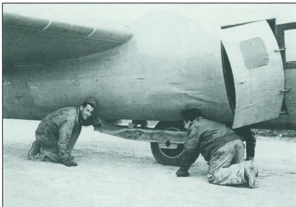
M/Sgts. Alvan H. Richardson and Bernard B. Cohen, engineers, examine German Heinkel bomber tail wheel installed on Lt. Alvin L. Nothesis' plane number 44-6606, 20th Squadron, by crew, Rumanians, and Russians, after original was lost to combat and emergency landing in Rumania. (Group Photo / W. Greenhalgh)
