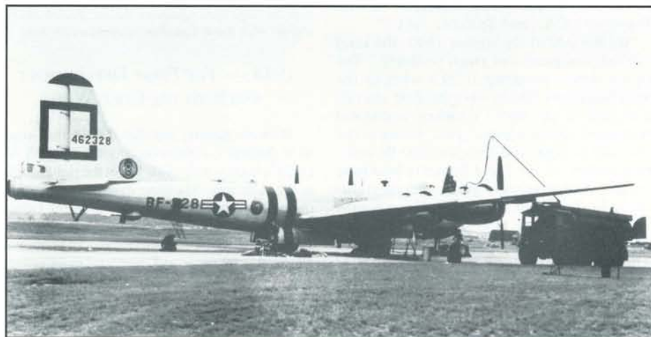
96th Squadron B-29-25-MO, s/n 42-62328, during deployment to RAF Lakenheath, August 1948. Note the RAF fuel bowser servicing the right outboard fuel tank. Later this aircraft served with both No. 149 and No. 4 Squadrons in the RAF. (Courtesy of the United States Air Force)
