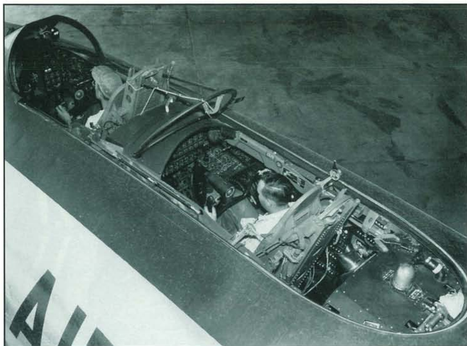
With the canopy removed, the compact tandem pilots' stations are visible. The copilot operated the fuel and communications panels from the right side console. The A-5 defensive fire control system was located behind the copilot whose seat rotated 180°. (Boeing Photo)
