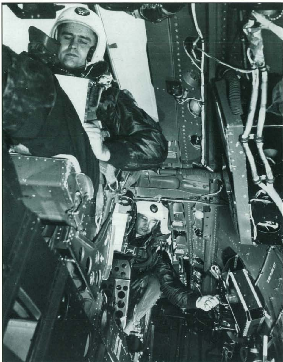
The pilots' seats in the B-47 were located above the catwalk. At the aft end of the catwalk was an access panel known as the hell hole through which the crew members would enter the bomb bay to practice in-flight arming of nuclear weapons (IFI/IFE). (Boeing Photo)
