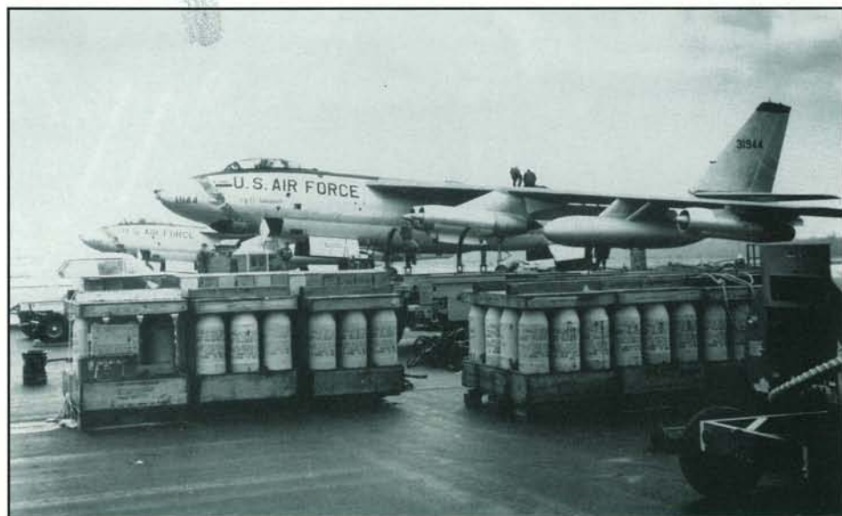
The City of Savannah was B-47E s/n 53-1944 assigned to the 2d Bombardment Wing. It had the partial white anti-radiation finish. Each of the pallets in the foreground held 32 RATO bottles used to boost the heavily loaded bomber off the ground. (Courtesy of Eighth Air Force Museum)
