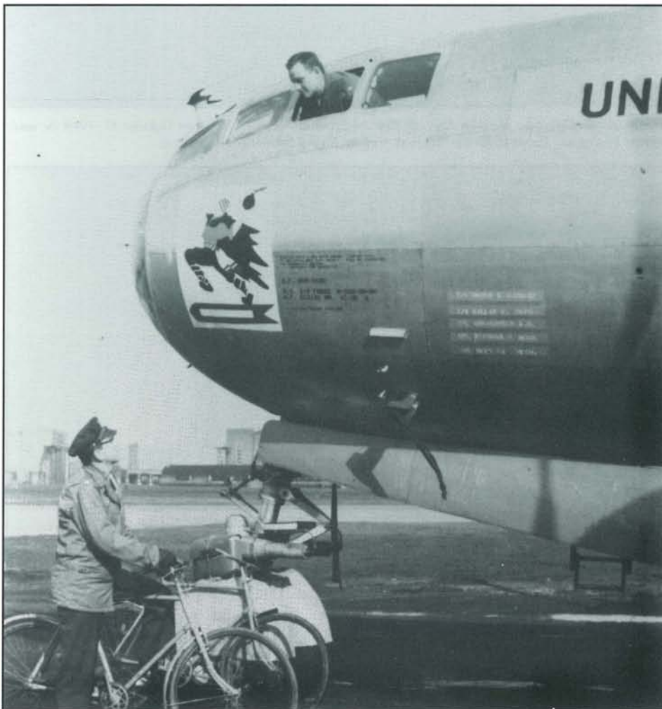
20th Squadron B-50A, 46-036 during deployment to England, February 1950. Note the nose wheel steering cylinders on the nose gear strut. (Courtesy of the United States Air Force)
