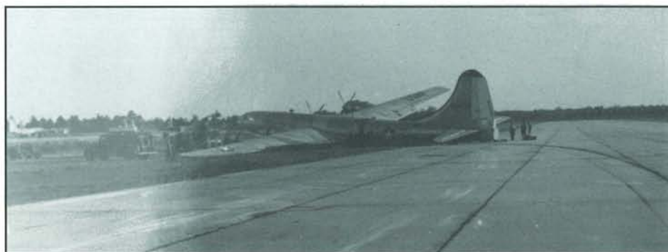
This is the 2nd Air Refueling Squadron's KB-29M, s/n 44-86280, that experienced a gear failure on landing at Chatham Air Force Base, April 3, 1950. (Courtesy of the United States Air Force)
