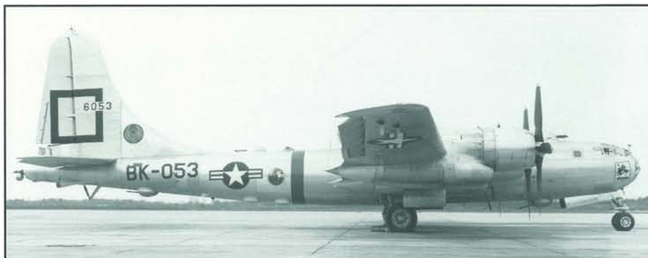
A 20th Squadron new B-50A at Andrews Air Force Base, Maryland, February 1949. Note Pineapple Pete insignia on the nose and green waist band. When the Triangle S markings were applied, the waist band color changed to blue. This aircraft was equipped for aerial hose refueling. The refueling receptacle appears aft of the tail skid. (Courtesy of S. Williams)
