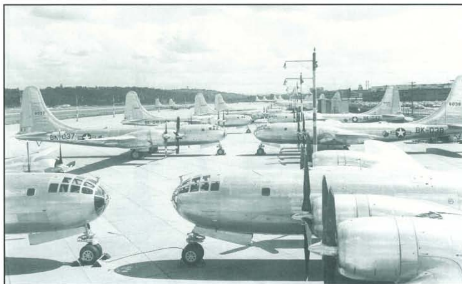
These B-50As on the flight line at Boeing Field, Seattle, bear a marked resemblance to their B-29 predecessors. Major externally visible differences include: nose wheel steering, Curtiss Electric propellers, huge Pratt & Whitney R-4360 engines in nacelles with recessed oil collar inlets, and the taller vertical tail. (Courtesy of S. Williams)
