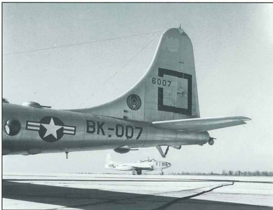
The tail of B-50A, 46-007, reveals its BK-007 buzz number, Eighth Air Force insignia on the fin fillet, and open square for the 2nd Bombardment Group. These aircraft were equipped with three .50 caliber machine guns in the tail and the AN/APG-15 gun-laying radar, as indicated by the suspended spherical antenna. (Courtesy of S. Williams)
