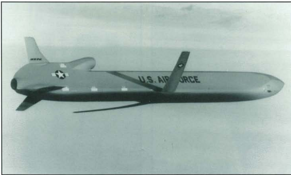
The AGM-89 Air-Launched Cruise Missile (ALCM) comes in two models. The AGM-89B nuclear weapon, and the AGM-89C conventional missile. This missile is shown in its flight mode with the wings spread and the engine inlet erected. Up to six of these missiles may be carried beneath each wing of the B-52s and another six on an internal rotary launcher. (Boeing Photo)
