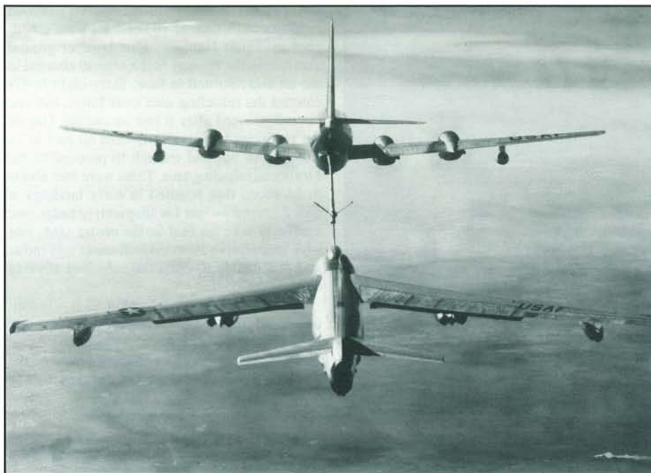
A B-47 takes fuel from a KC-97. Note how the wings on both aircraft are bent upwards under normal 1-g flight loads. The B-47 has added a bit of flaps to slow down behind the lumbering tanker. (Courtesy of the United States Air Force)
