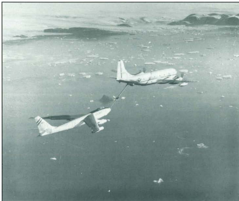
This unusual photograph shows two 2d Bomb Wing aircraft performing a low-level refueling demonstration during deployment to Ramey AFB, Puerto Rico in February 1961, as part of Exercise BLUE BANNER. To perform such an operation at low level required the crews to be very experienced, and the aircraft extremely light. Usually little or no fuel was transferred. (2d Bomb Wing History)
