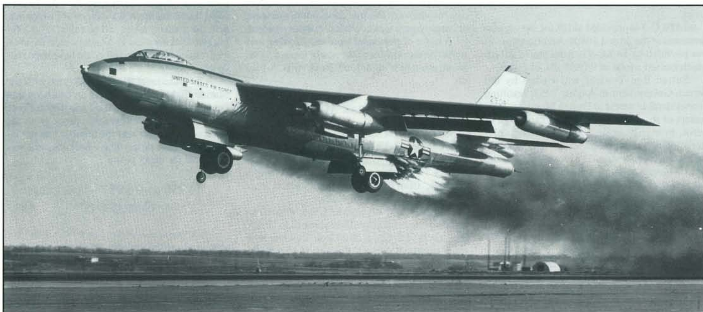
Belching fire and smoke from its belly, this B-47E was making a RATO takeoff. These bottles would be dropped in a clearway at the end of the runway. (Boeing Photo)
