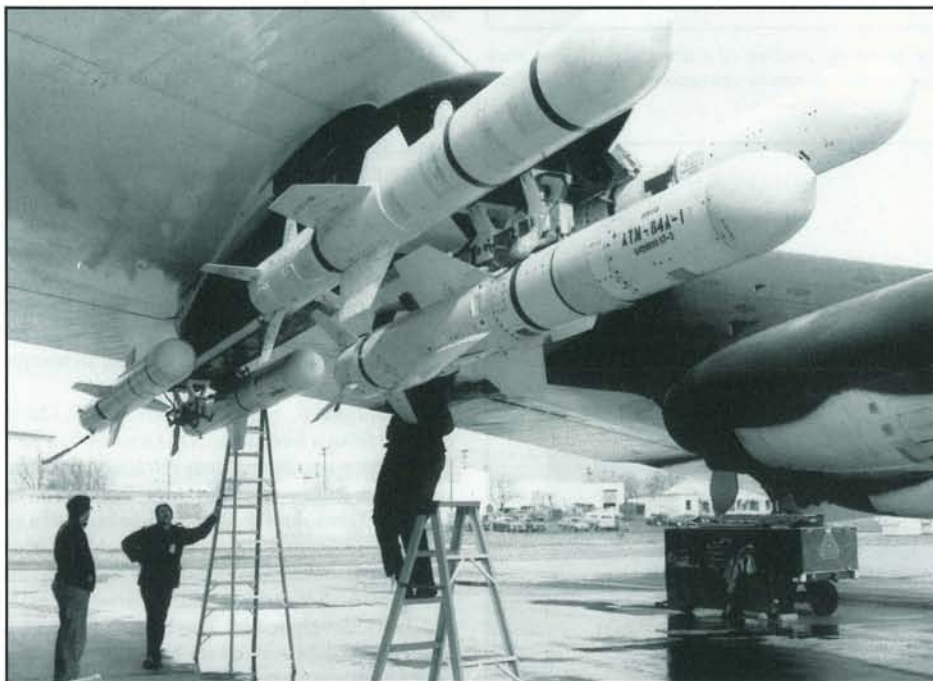
These are ATM-84A training missiles used to simulate the AGM-84A Harpoons carried on the external pylons of the B-52Gs and later the B-52Hs. Originally, six missiles were carried on each pylon; however testing proved that four was the optimum number to be carried. (Courtesy of the United States Air Force)
