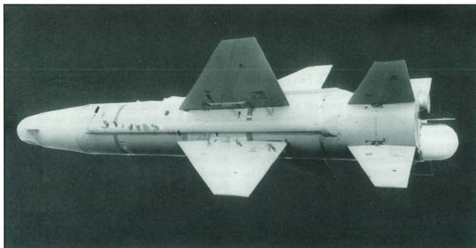
This is an AGM-142A Have Nap missile with its bulbous TV data link antenna mounted on the rear end. (Courtesy of Lockheed-Martin)
