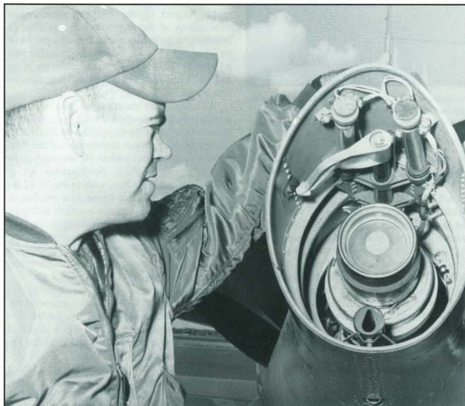
T/Sgt. Thomas "Obie" O'Brien inspected the working end of the KC-97 boom when he came to Boeing in Seattle for a delivery flight. A pair of boom lights may be seen at the top of the boom shroud. (Courtesy of Thomas "Obie" O'Brien)
