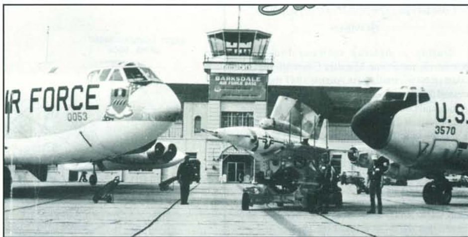
These stable mates were assigned to the 2nd Bomb Wing at Barksdale AFB during the mid- and late 1960s - The Corogard-finished B-52F-110-BO, s/n 57-053 in yellow, with its white anti-radiation lower surfaces, a pylon-mounted GAM-77/AGM-28 Hound Dog missiles, and the KC-135A-23-BN, s/n 62-3570, also in the Corogard finish. This photograph was taken in front of Barksdale Base Operations. Note the ornate scallops on the 2nd Bomb Wing insignia. (Courtesy of the United States Air Force)
