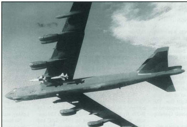
The 49th Test Squadron tested the AGM-142A Have Nap stand-off missiles on B-52G-90-BW 57-6520 from the 2d Bomb Wing. Two missiles are mounted on the left pylon, while a data link sensor is installed on the right pylon. (Courtesy of Lockheed-Martin)
